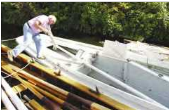
Angus Houstone living typically dangerously, 'aboard' a pair of traditional 40' working Sharpies at The Centre for Wooden Boats, Seattle. Note the lack of cabin, low sides and narrow side decks. (I am not referring to Angus)'.
