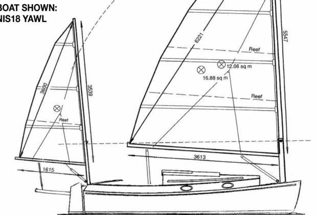
The sails remain on the boom and in the case of the 18, 23 and 26, may remain packed down in the mast track as well. So, in one action, booms, sails and masts are packed away. No junk on the cabin roof, all is ready for trailing.
