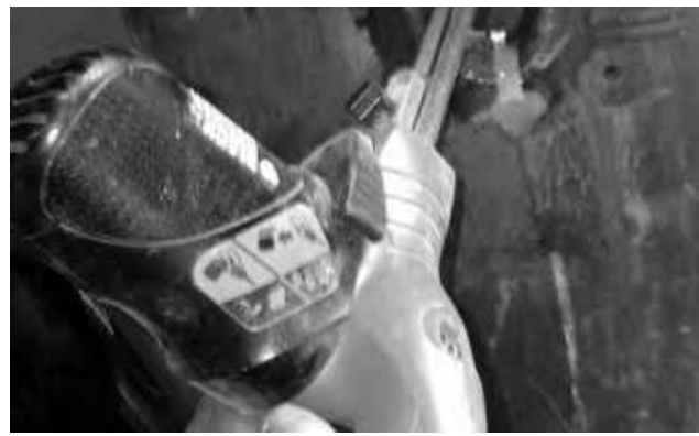
The Black & Decker Powerfile showing custom dust extraction adapter.
